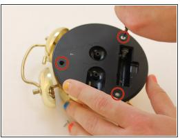
Using a Phillip's Screwdriver, remove the three screws on the back cover of the clock.
