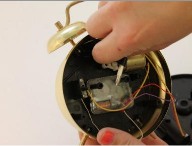
Using your fingers, remove the bell hammer from the inner apparatus of clock.
