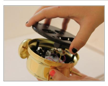
Using your hands, remove the back cover of the clock by grasping it and pulling it upwards.
