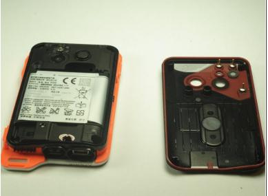
Remove the battery shield with the plastic opening device.
