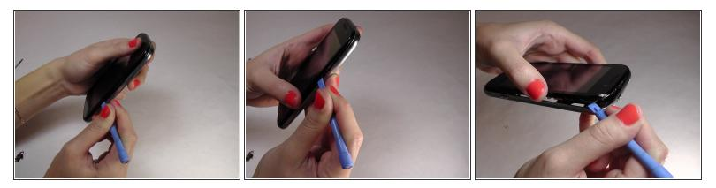
• Wedge the flat end of the spudger between the mid frame and the digitizer.
