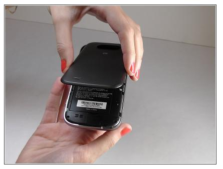
• Remove the back cover of the phone to expose the phone's mid-frame.
