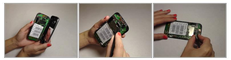
• Gently pry the mid frame away from the rest of the phone to expose the motherboard.
