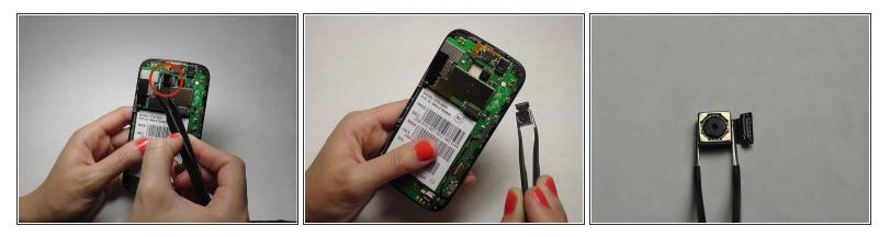
Use the tweezers to grip the back facing camera. Gently pull until the camera is completely removed from the motherboard.
