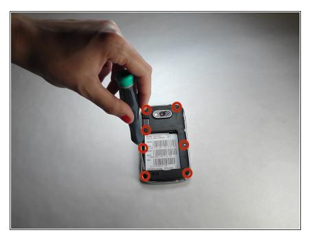
Use the Phillips Head 00 screw driver to unscrew the seven 0.1mm screws along the perimeter of the phone's mid frame.
