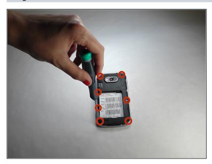
Use the Phillips Head 00 screw driver to unscrew the seven 0.1mm screws from the phone's mid frame.
