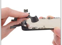
• Carefully peel the cable assembly off of the LCD shield plate to remove it from the display.
