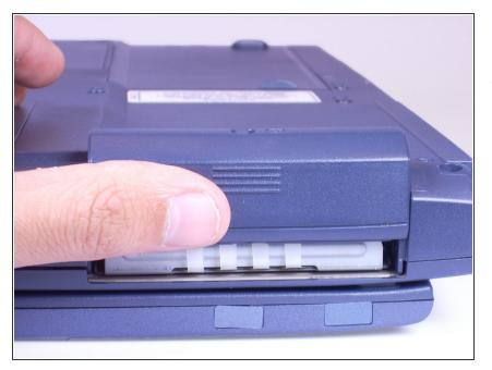
Placing your finger on the raised grip, push up on the hard drive cover. This will remove the hard drive cover from the laptop.
