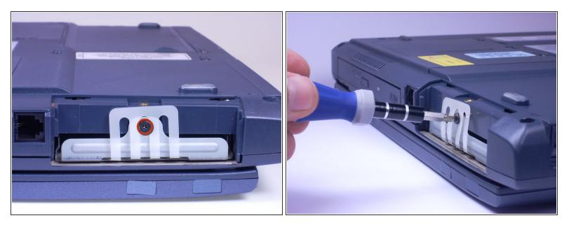
Using a Phillips screwdriver, unscrew and remove the screw surrounded by the white plastic.
