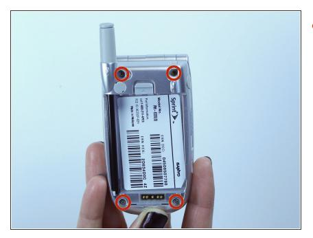
Unscrew all four, 5mm Tri-Wing screws.
