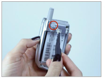
Use a push pin or tweezers to remove the neoprene screw-cover located on the upper, left corner of the back casing.
