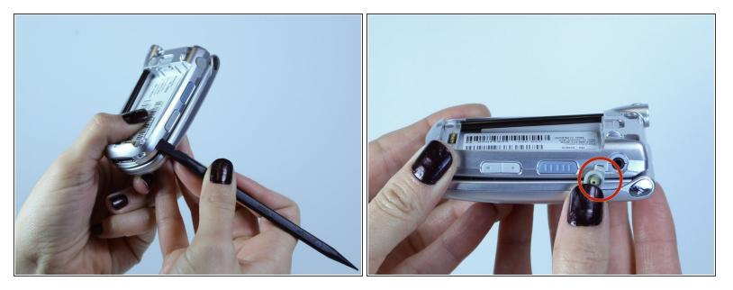
• Pry the back casing off the device using a spudger. Work your way along the edges to completely separate the back casing from the device.
