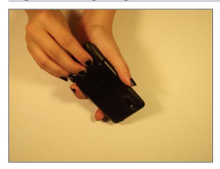
Use fingers on either end of the button edges of the phone to pull back cover off. It should slide off.
