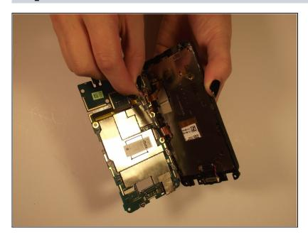
Disconnect the two aluminum flex cables
