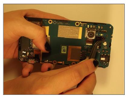
Unplug the wire connecting the vibrator to the board with your tweezers
