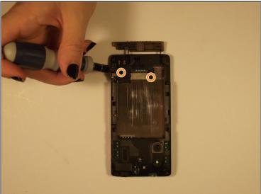
• Remove the two revealed screws on the outside (Torx = red, Phillips = orange), and then remove the two phillips on the bottom of the phone
