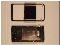
• To remove the remaining cover, lift the side port, which was previously uncovered, then lift the outer shell from the bottom of the phone and slide it forward
