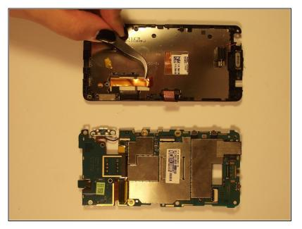
The flex cables should be the only binding and after being removed should leave you with the separate screen
