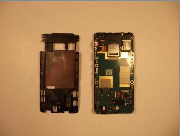
• Remove the rear housing by prying around the edge with your Safety Pry Tool
