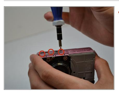
Remove the three screws from the bottom of the camera.
