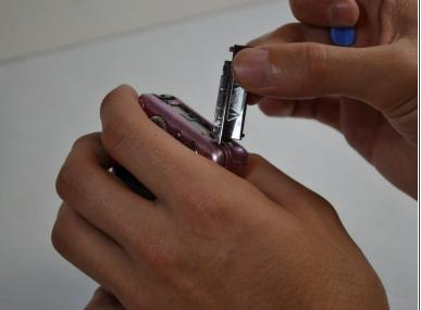
• Using a plastic opening tool, gently lift the side of the silver piece on the right side of the camera until it can be removed.
