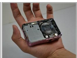
Use a plastic opening tool to separate the front case of the camera, and gently remove it.
