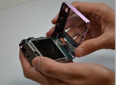
Carefully remove the back case with a plastic opening tool.
