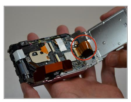
Lift the display from the rest of the camera and gently separate the connecting tape using tweezers.
