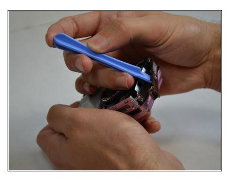
Use a plastic opening tool to remove the silver piece on the left side of the camera.
