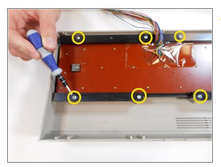
3. Remove eight 6.75 mm ph2 screw heads to detach the keyboard face from the front casing. (Two remaining screws on the right side.)
