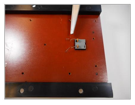
6. Next, carefully cut the two small wires which are connected from the Shift/Lock key to the keyboard.
