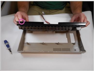
7. Turn the keyboard down on its face and push the shift lock key out from the back of the keyboard.
