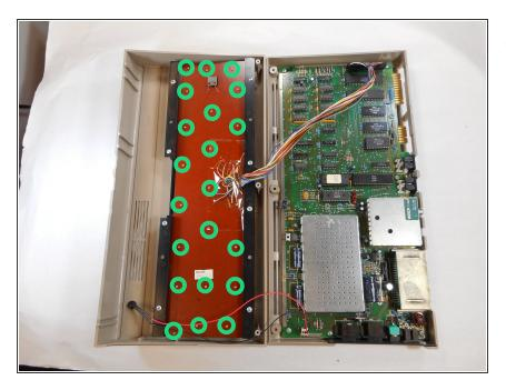
4. Remove twenty-three 3.38 mm ph2 screw heads from the back of the keyboard facing
