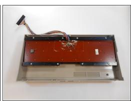
• 5. Detach the multi-colored wire bundles connected to the motherboard
