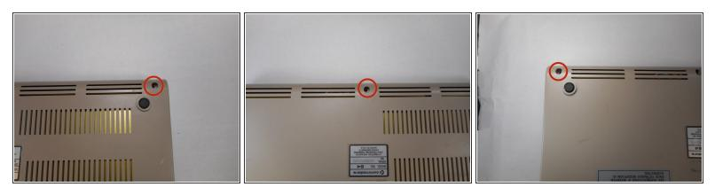
1. Remove three 6.75mm ph2 screw heads from the casing
