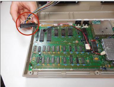
1. Detach the multi-colored wire bundles that's connected to the motherboard
