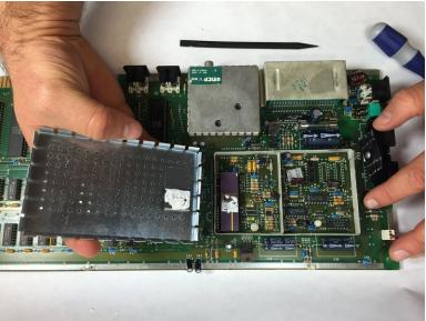
2. Without using any tools prop up the metal VIC plate with both hands to expose the VIC chip.
