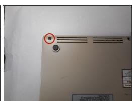
1. Remove three 6.75mm ph2 screw heads from the casing
