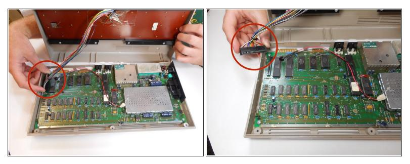
1. Detach the multi-colored wire bundles connected to the motherboard.
