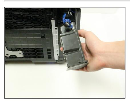
Rotate the AC adapter toward you so that the blue cord, with white connector head, is facing you.
