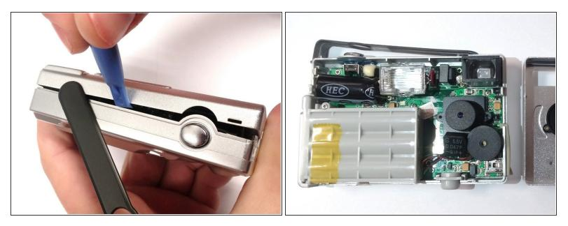
Using a prying tool or fingernail, gently separate the back plate from the front plate, exposing the inside of the camera.
