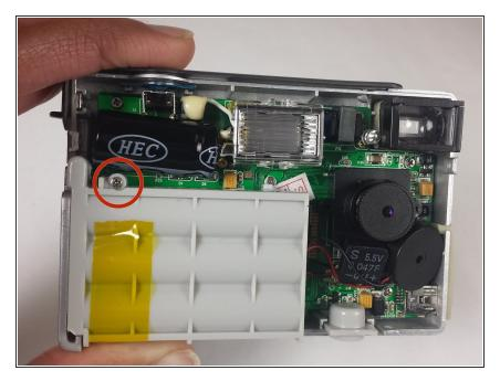
• Remove the 4.5mm screw with the iFixit ph#00 screwdriver
