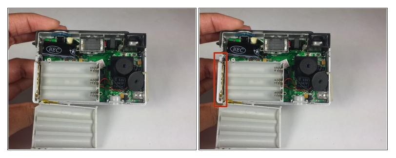
With your fingers, gently pull the two pieces of the battery case apart. At this point, the battery door should be exposed
