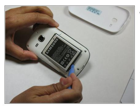
Use your thumb nail or the plastic opening tool to lift the battery out of the device.
