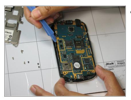
Use the plastic opening tool to lift the motherboard out of the device.
