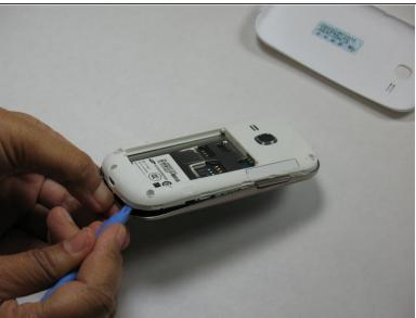
Use the plastic opening tool to pry into the bezel to separate the mid-frame from the device
