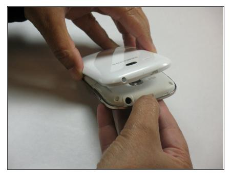
Make sure that the phone is turned off. Then use your thumb nail or a plastic spudger to pry open the back cover.
