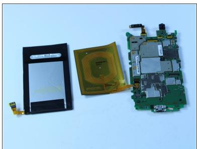
A Carefully peel back the orange adhesive from the battery. Make sure to remove all the adhesive attaching the battery to the motherboard.
