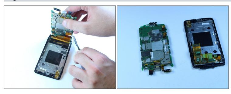
• Carefully use the <u>tweezers</u> to separate the motherboard from the screen.
