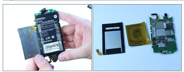
⚠ Carefully peel back the orange adhesive from the battery. Make sure to remove all the adhesive attaching the battery to the motherboard.
