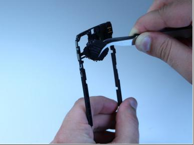
Use the tweezers to gently push the loudspeaker out of the housing frame.
