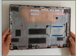
• Starting from the SD Memory Card hole, start prying between the top and bottom cases.
