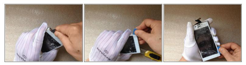
With a cutter, make a room for a plastic tool, then continue with separating the Touchscreen & LCD Display from the frame.
