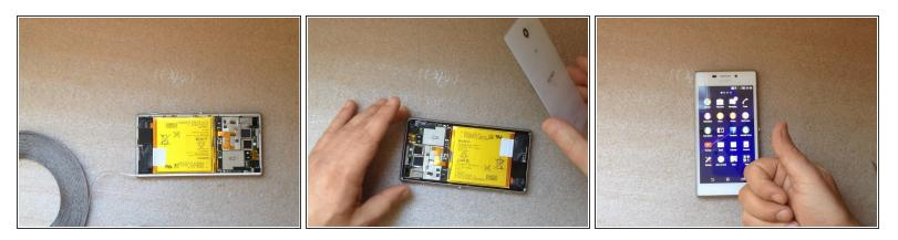
• When finishing the assembly of the inner parts, use same technic to install the Back cover.
