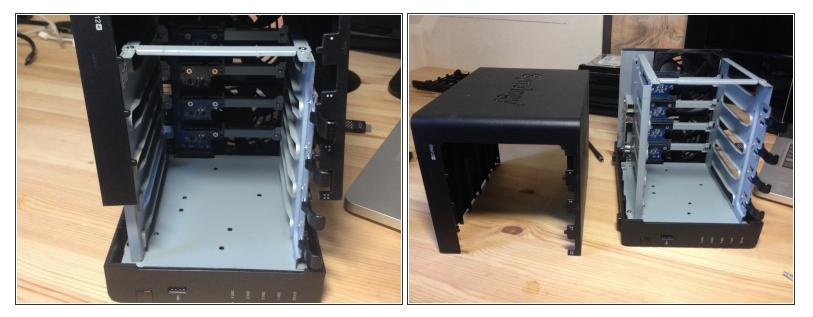
With the NAS on its right side, lift up the enclosure, mind the tabs on the top of the case.
