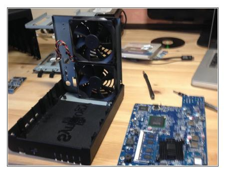
Starting from the front of the unit, remove the motherboard from the unit.
