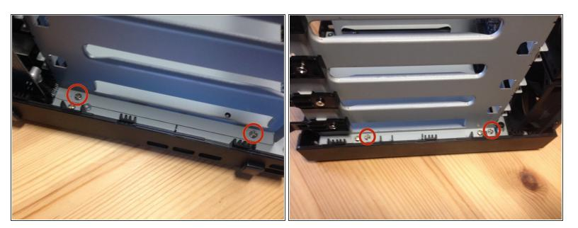
Remove the four screws securing the HDD bays
