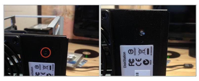
Remove the screw securing the HDD bays enclosure.
