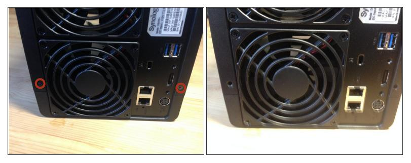
Remove the two screws in the back of the NAS, on the top and bottom.
