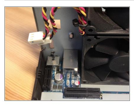
Remove the I/O board by lifting it up
