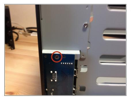
Remove the screw securing the I/O board.
