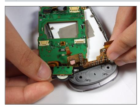
• Pull/pivot the LCD main board as shown in order to remove.
