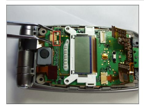
Unlock the minor LCD connector by applying bilateral pressure with tweezers, as shown.
