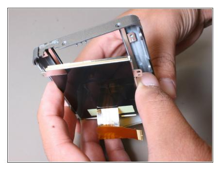
• Remove the LCD screen from the remaining casing of the camera.
