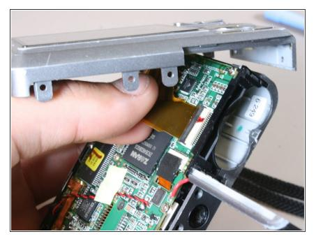
Gently pull the ribbon away from the motherboard. This will allow the cover to separate from the rest of the camera.
