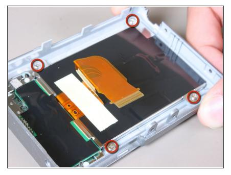
Locate the four screws in each corner of the LCD screen and carefully remove them. After they have been removed, ensure the screws stay separate from the 3mm case screws.
