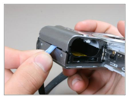
Slide the battery door open and slightly open the side of the case with a plastic opening tool.
