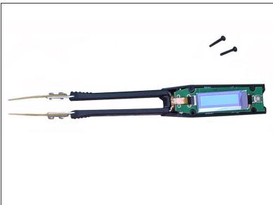
Start by removing the 4 screws in the back of the device using a size 00 Philips screw driver.
