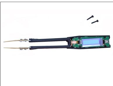
Start by removing the 4 screws in the back of the device using a size 00 Philips screw driver.
