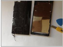
Continue separating the display from the frame by using plastic opening tools.
