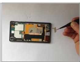
Remove the Loudspeaker metal bracket.
