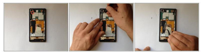
• Unscrew the screw and remove the Wi-Fi Antenna.
