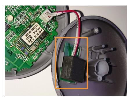
when reassembling take care to stick the NFC tag to the correct location in the cover
