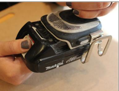
Push down on the button on the front of the battery and slide the battery forward.
