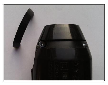
The last 2 screws are hidden under a small plastic cover at the bottom of the motor block.
