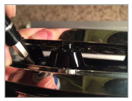
Insert a strong spudger or flathead near the riser and gently pry until the plug starts to come out. Work your way around to loosening each one.
