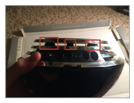
Locate the 3 risers the hold the base plate in place
