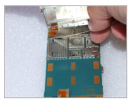
Carefully open the LCD and keyboard assembly, and remove keyboard connector.
