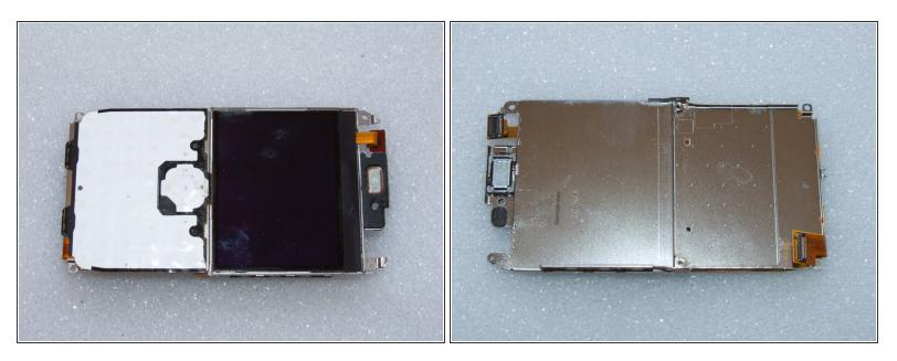
• Both sides of the LCD and keyboard assembly removed.
