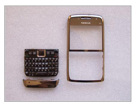
• Front cover, rubber keyboard and bottom cover removed.
