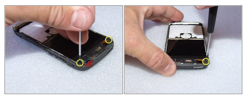
• Remove these two Torx T6 screws at top of the smartphone.
