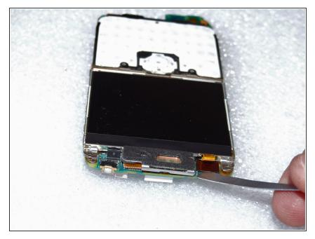
• Remove the LCD connector.
