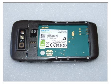
• First remove back cover, battery, chip and memory card .
