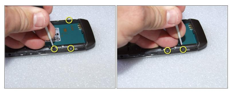
• Press these four latches (each side has two) to open front cover.
