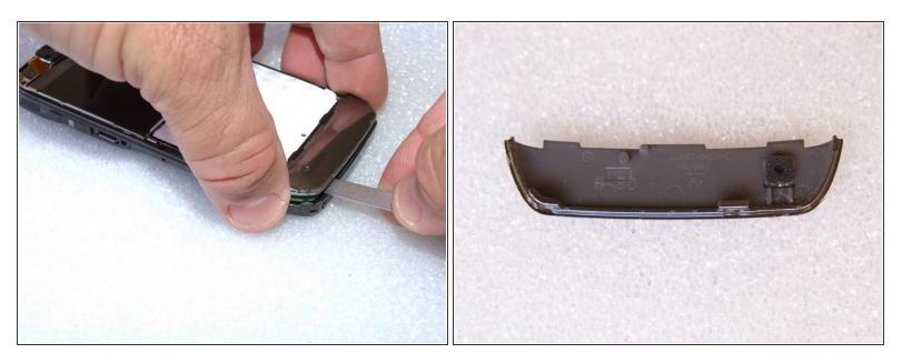
• Carefully remove the bottom cover. This cover has no screws, only latches.
