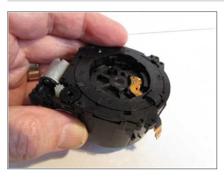
Note: from here on reassembly is critically dependent on the correct alignment of parts. It is highly recommended that you practice disassembly and reassembly of each stage several times before going on to the next.
