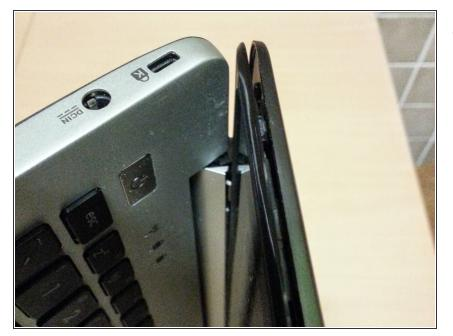
For a couple of months I was hearing some cracking when opening my laptop but never paid much attention. Big mistake. The left hinge was getting stuck, twisting the plastic cover corner to its limit. Until the hinge completely blocked today and the screen top snapped and slightly opened, as you can see in the picture.
