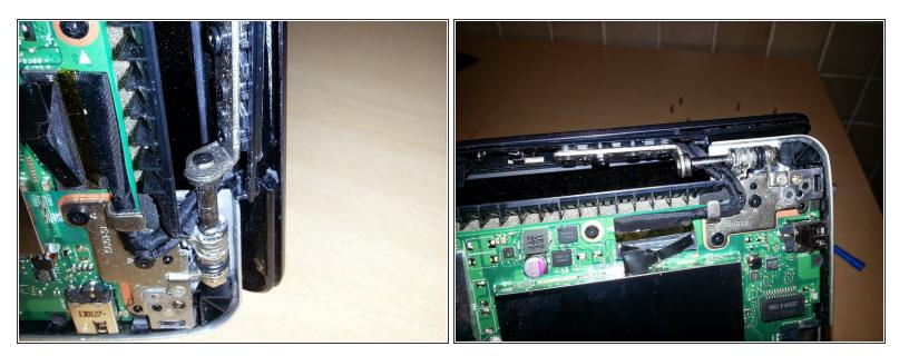
• Now I can see the hinge that is causing the problem and the broken plastic around it.
