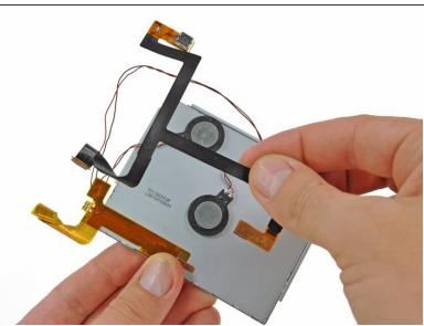
Lift the camera ribbon cable up off the upper LCD, minding any adhesive that may still be attached.
