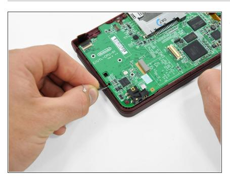
Deroute the microphone and antenna cables through the slot in the motherboard.
