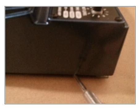
To separate the enclosure parts, use a small screw driver as a lever.
