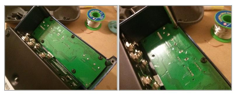
Slide the top part of the enclosure enough to access the five screws that you'll need to remove.
