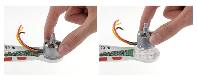
• Remove the motor from the Phantom.
