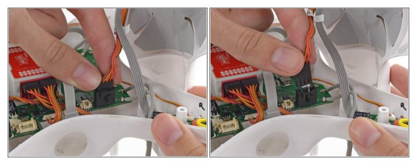
• Lift the GPS cable molex connector up out of its socket on the main board.
