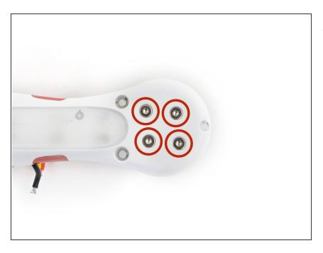
• Unscrew the four 2 mm motor hex bolts from the case bottom shell.
