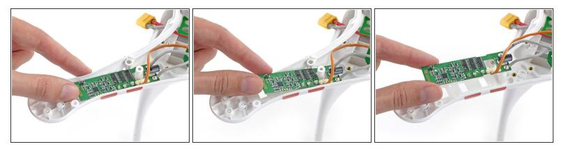
• Remove the ESC from the Phantom.
