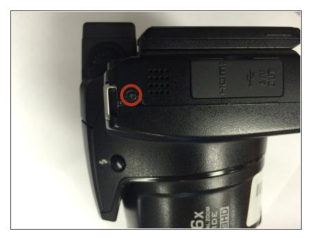
On the right side of the camera, remove the first visible screw above the HDMI and A/V OUT cover.
