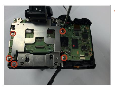
Remove the five indicated screws that are attached to the metal plate.
