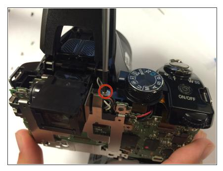
Remove the hidden top screw that is attached to the metal plate.
