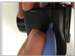
Use a plastic iFixit opening tool to gently loosen the top and sides of the camera.
