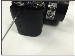
On the left side of the camera, use a Phillips #00 Precision Screwdriver to remove the two marked screws.
