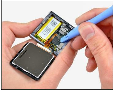
Use an opening tool to disconnect the display data and digitizer cable connectors up from their sockets on the logic board.
