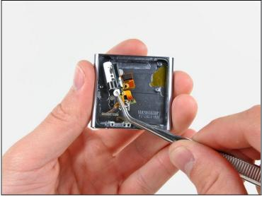
• Use a pair of <u>tweezers</u> to carefully pull the headphone jack toward the center of the Nano.
