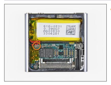
Remove the single 1.9 mm Phillips screw securing the logic board to the outer case.
