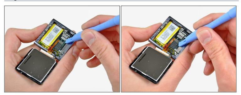
• Use an opening tool to disconnect the display data and digitizer cable connectors up from their sockets on the logic board.
