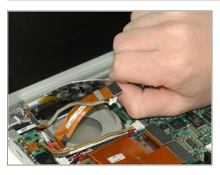
Lift the left fan out ofo the computer (the yellow tape will peel up with the fan).
