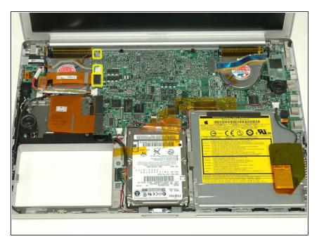
Disconnect the fan, inverter, and DC-In cables from the right side of the fan.
