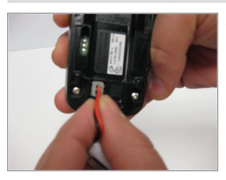
Remove the red-and-black-wired port from the plug directly under the battery compartment.
