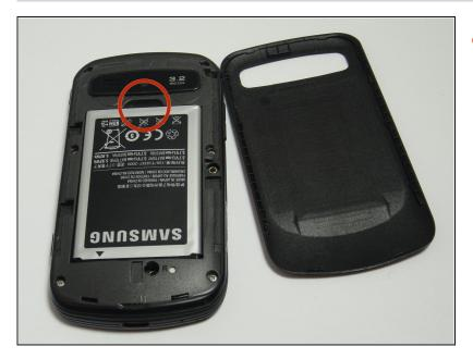
Place your fingernail or plastic tool into the hole beneath the camera and carefully lift out the battery.
