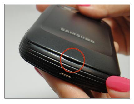
Slide your fingernail or plastic opening tool under the slit and pull the cover up.
