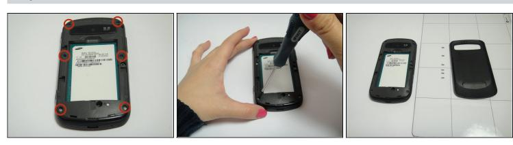
• Use a Phillips #00 precision screwdriver to remove the six screws from the back of the phone.
