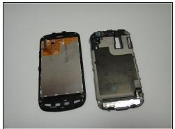
• Pull back on the five clips on the sides of the phone to remove the shield.
