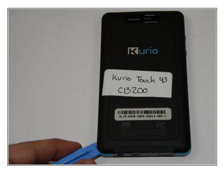
Make sure to open the back cover easily using the plastic opening tool.
