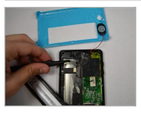
Remove the plastic cover that is covering the camera area using tweezers.
