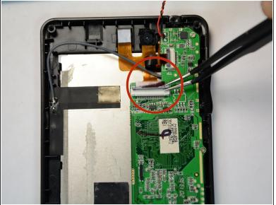
• Remove the copper wires by using the Tweezers to replace your new camera.
