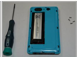
To remove the battery, make sure the four 5mm Philips screws on each side of your device is open using the philips#1 Screwdriver.
