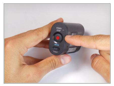
To access the memory card, push left on the rear of the Action Cam.
