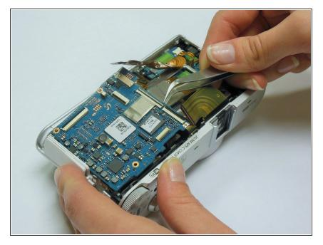
• The motherboard is now free. Pull the motherboard up and slightly away from the input compartment; it will lift out easily.
