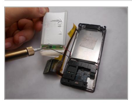
Use a soldering iron to remove the wires from the red and the black terminals.
