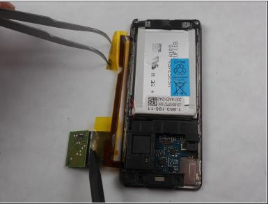
Peel back the layer of tape along with the processor, which is located just below the battery, using the tweezers and the spudger.
