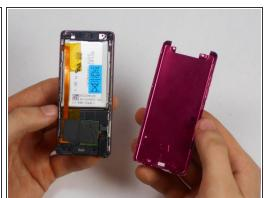
Remove the back plate from the device.
