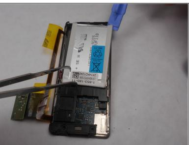
Slide a prying tool underneath the top portion of the battery and lift it from the case.
