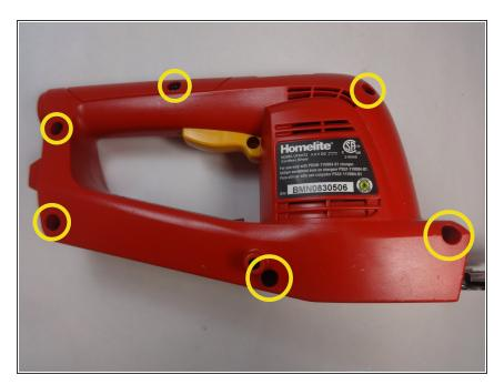
Use a Philips-head screwdriver to remove the six, 15 mm screws from the casing.
