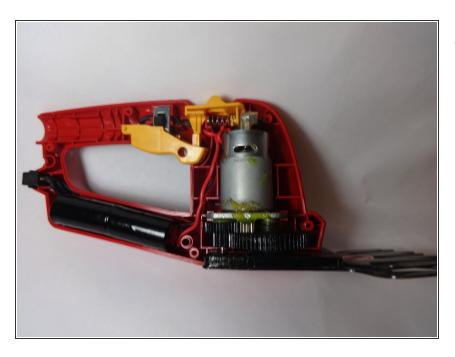
Remove the faceplate from the main body of the device, lift it and expose the inner mechanisms.
