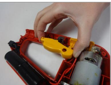
Locate and remove the operating switch from the device.
