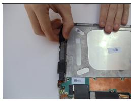
• Remove the two 4 mm screws from the right side of the housing with the Phillips #00 screwdriver.
