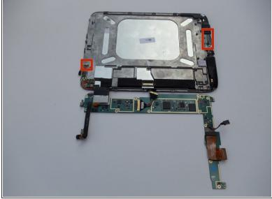
Pull up the L-shaped board to disconnect the two connectors at the top and bottom of the board.
